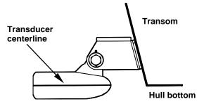
Align transducer centerline with hull bottom.
